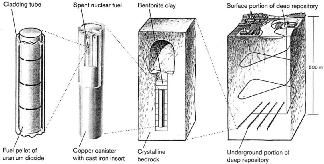
Fig. 1. The KBS 3 concept for disposal of spent nuclear fuel.
