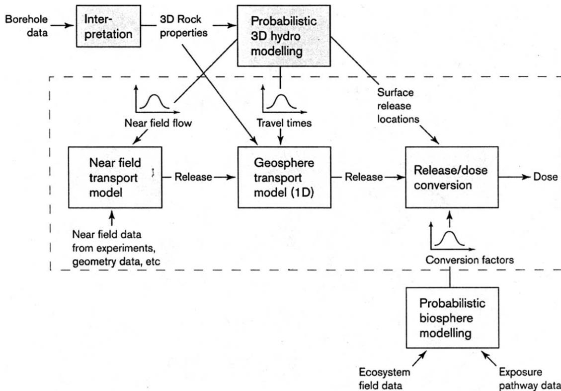
Fig. 2. Overall structure of data and models. The probabilistic transport modelling discussed in this paper is enclosed by the dashed line. The figure illustrates how several crucial input distributions are determined through separate hydrological and biosphere modellings.
