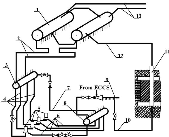
Fig. 1. Schematic representation of one loop of the RBMK-1500 MCC: (1) drum separator; (2) downcomers; (3) MCP suction header; (4) MCP suction piping; (5) MCPs; (6) MCP discharge piping; (7) bypass line; (8) MCP pressure header; (9) GDHs; (10) lower water communication line; (11) fuel channel; (12) steam–water communication line; (13) steam lines.
