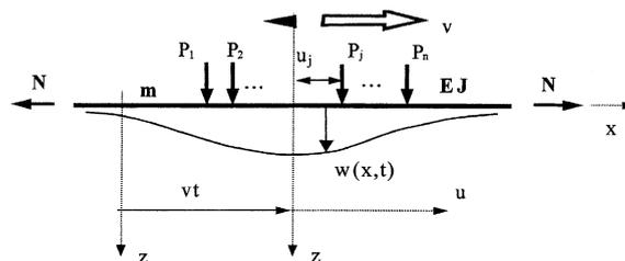
Fig. 1. Model of track structure with load.
