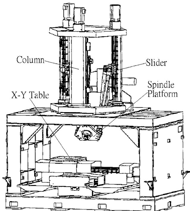
Fig. 1. Structure of the serial-parallel type machine tool.
