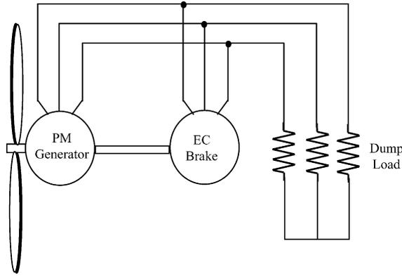
Fig. 1. Configuration of the wind turbine electric part in case of grid connection loss due to fault (PM generator supplying the eddy current brake and the resistive dump load).
