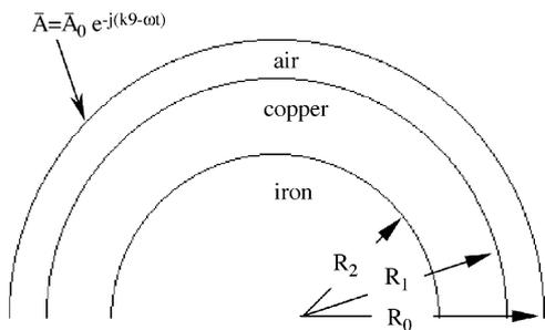
Fig. 2. Geometry of the non-salient solid iron rotor structure surrounded by a sinusoidal rotating magnetic field.
