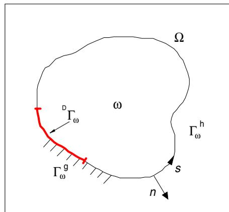
Fig. 1. A two-dimensional problem with the domain of interest  $\omega$  embedded in a fictitious domain  $\Omega$  ( $\Gamma_\omega^g$ : boundary under kinematic constraint,  $\Gamma_\omega^h$ : boundary under natural condition,  ${}^D\Gamma_\omega$ : design boundary).
