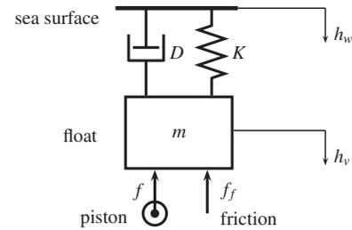
Fig. 2. A mechanical circuit representation of the point absorber.
