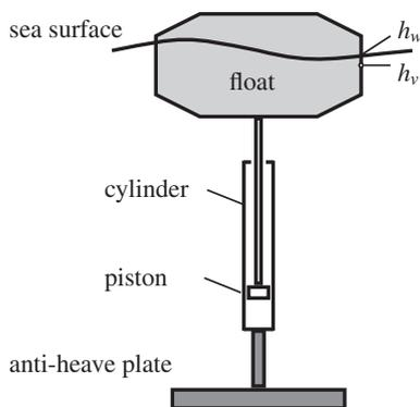
Fig. 1. Schematic diagram of the point absorber.
