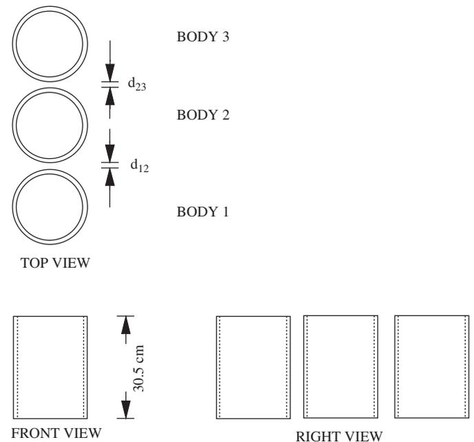
Fig. 2. Three cylinder test geometry: (M–M–M).
