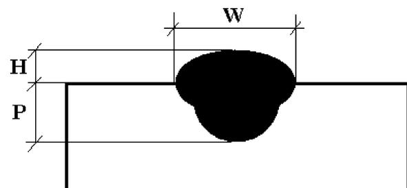
Fig. 1 – A schematic representation of weld bead geometry parameters ( $W$ : width,  $H$ : height,  $P$ : penetration).
