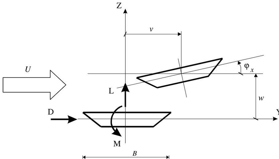
Fig. 2. Aeroelastic forces on a bridge deck.
