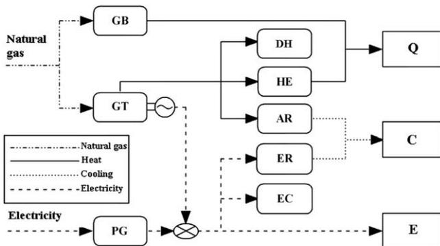
Fig. 1. Schematic diagram of gas turbine cogeneration system.
