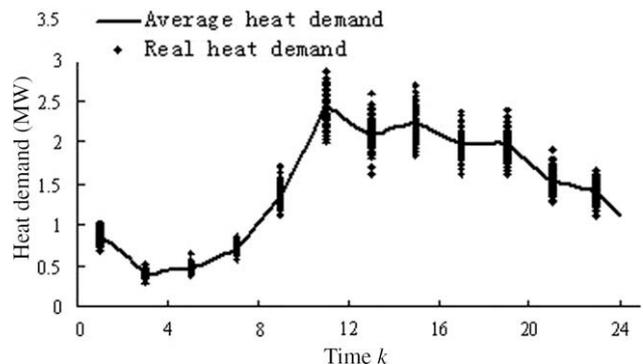
Fig. 2. An example of real data of the heating demands.
