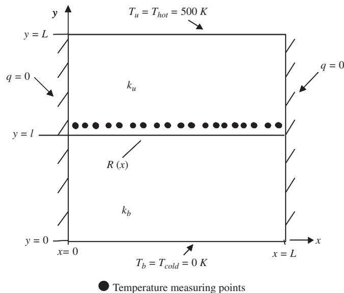
Fig. 1. Illustration of the model of a simulated steady-state experiment to retrieve thermal contact resistance.
