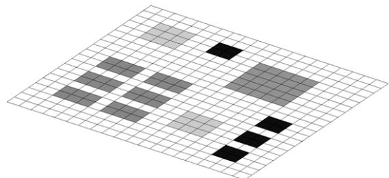
Fig. 4. Example of a locally smeared FE model of a PCB, the shaded locations are intended to model the effects of components and have increased stiffness and density compared to the underlying PCB (non-shaded).
