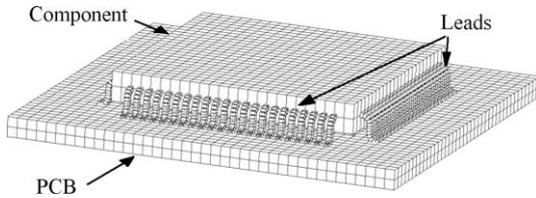
Fig. 1. Example of a detailed FE model of an individual component, a detailed model of a PCB would incorporate several of these and other components over its surface.
