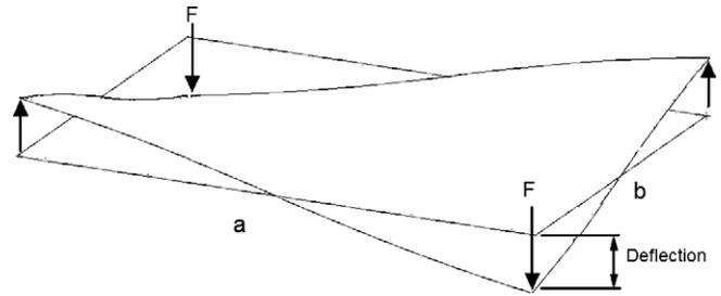
Fig. 3. Method of testing torsional stiffness of a component sample. Loads are placed on diagonal corners and the deflection is measured at the corners.
