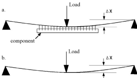
Fig. 2. Method of creating effective stiffness. An attached component specimen is either modelled or experimentally tested and the deflection measured (a), a FE model of an unpopulated PCB can be given an artificially high Young's modulus to give the same deflection and therefore effective stiffness as the real specimen (b).
