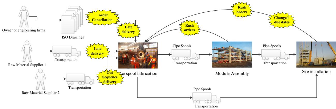
Fig. 1. Disturbances from piping supply chain of an industrial construction project.
