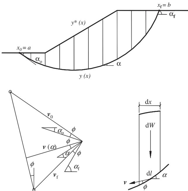
Fig. 1. Collapse mechanism, typical slice, and hodograph of the movement.
