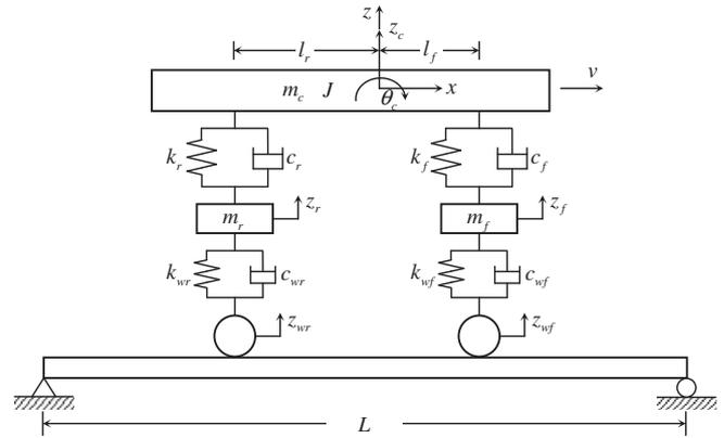
Fig. 1. Coupled vehicle–bridge model.
