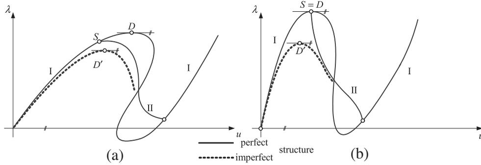
**Fig. 1.** Sketches illustrating the improvement of the prebuckling behavior accompanied by a deterioration of the postbuckling behavior of a perfect structure, and its influence on an imperfect structure (a) at the start and (b) at the end of the variation of a design parameter (hilltop buckling). (I: primary (prebuckling) path, II: secondary (postbuckling) path).
