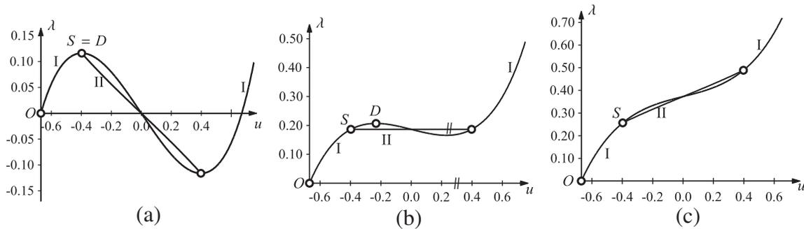
**Fig. 2.** Improvement of the prebuckling behavior accompanied by improvement of the postbuckling behavior of a perfect structure (a) at the start (hilltop buckling), (b) at zero-stiffness postbuckling, and (c) at the end of the variation of a design parameter. (I: primary (prebuckling) path, II: secondary (postbuckling) path).
