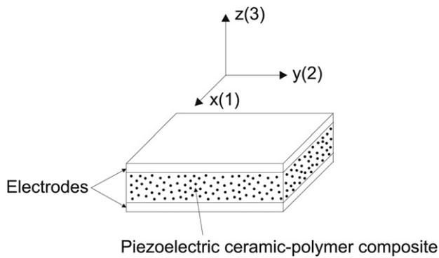
Fig. 1. Schematic of a piezoelectric paint sensor.
