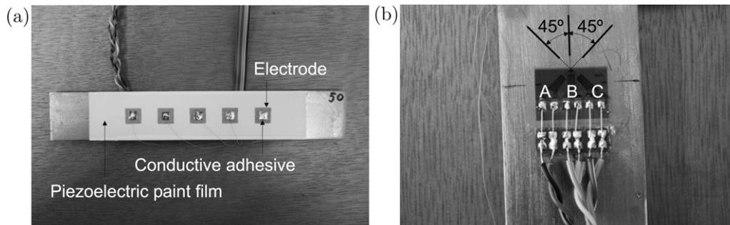
Fig. 3. Sample used in experimental tests: (a) top surface of the sample with five piezoelectric paint sensors, (b) bottom surface of the sample with a 45° rosette strain gauge.
