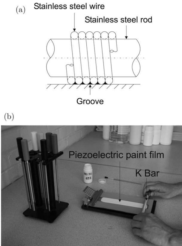
Fig. 2. K hand coater used to spread piezoelectric paint on the substrate: (a) schematic of a wired K bar, (b) substrate covered with a piezoelectric paint coating.
