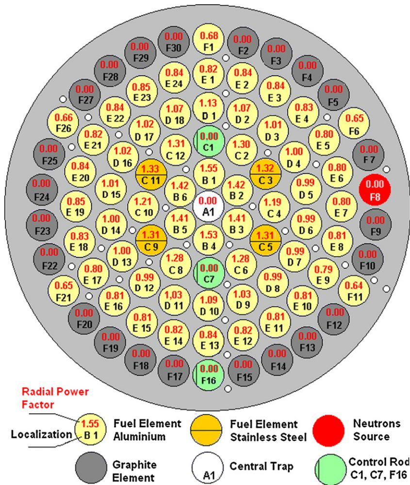
Fig. 1. Radial relative power distribution. (For interpretation of the references to color in this figure legend, the reader is referred to the web version of the article.)
