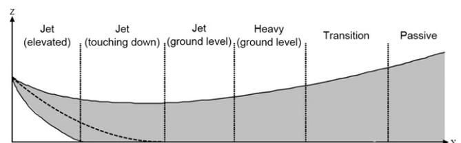
Fig. 1. Dispersion phases according to the UDM (case of heavy-gas behavior). (-----: centerline of the cloud, wind direction according to x).
