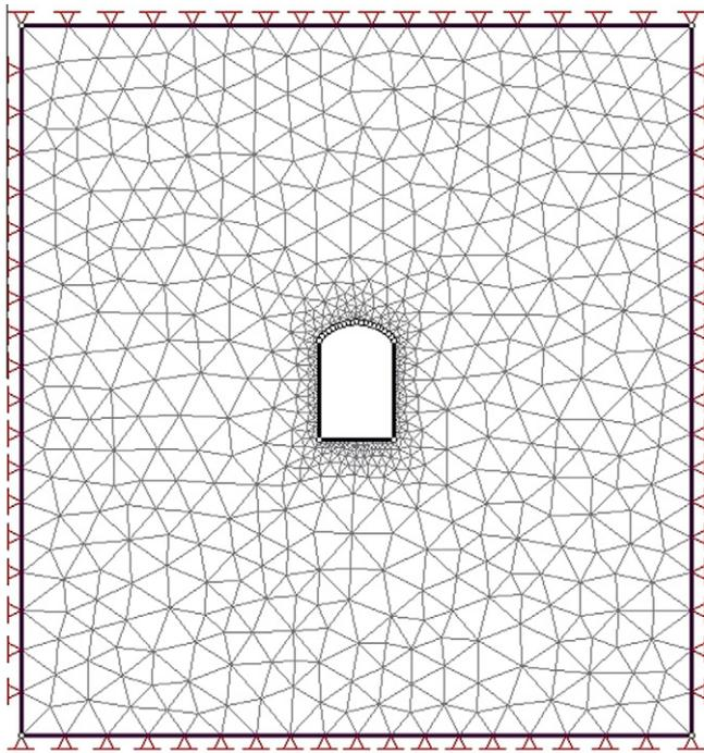
Fig. 1. Cavern of 33 m × 52 m cross section.
