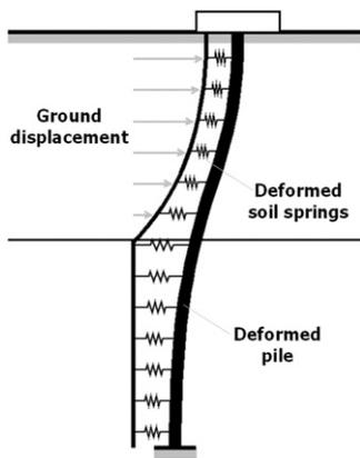
Fig. 1. Conceptual illustration of the displacement-based beam-spring model of the soil-pile system.
