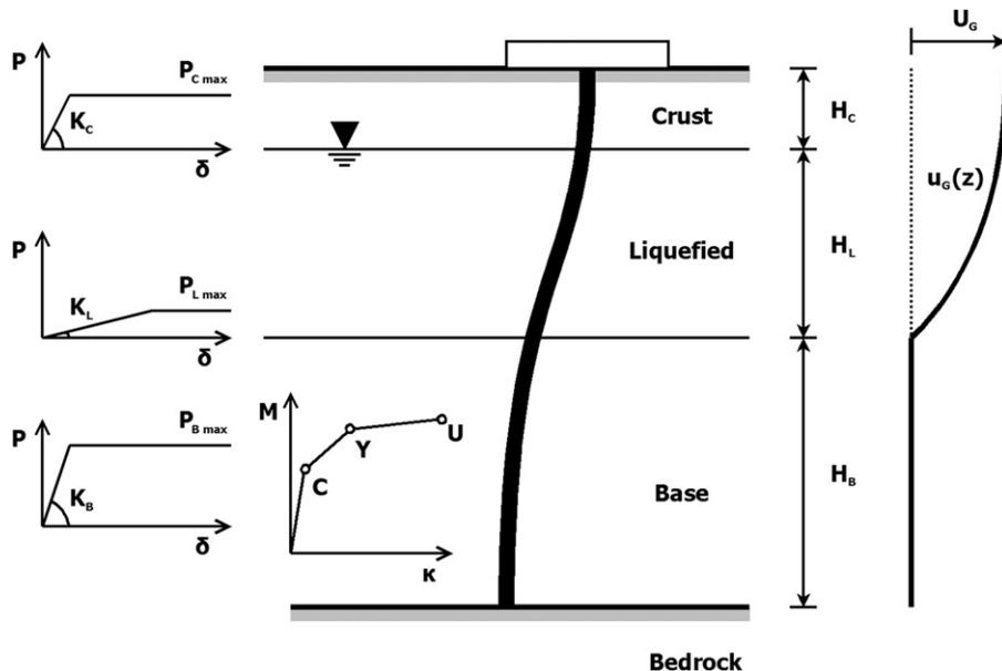
Fig. 2. Illustration of the various beam and spring properties of the adopted pseudo-static model.
