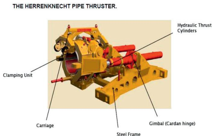
Figure 1. The *Directpipe* machine: Pipe Thruster
