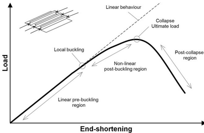
Fig. 1. Typical behaviour of a stiffened panel subjected to longitudinal compressive loads (adapted from Ref. [7]).
