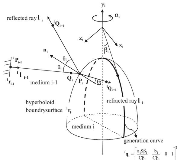
Fig. 1. A surface of revolution forms one boundary surface of a medium; schematic diagram of skew ray tracing at the boundary.
