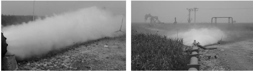
Fig. 1. CO<sub>2</sub> outflow and dispersion during pipeline decompression courtesy of Dalian University.
