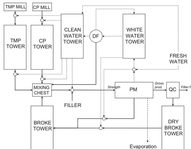
Fig. 1. Schematic flowsheet of a paper mill. The largest volumes and most critical unit operations are depicted and modelled.
