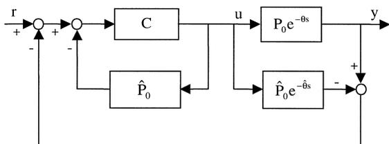
Fig. 1. A standard form of Smith predictor controller.
