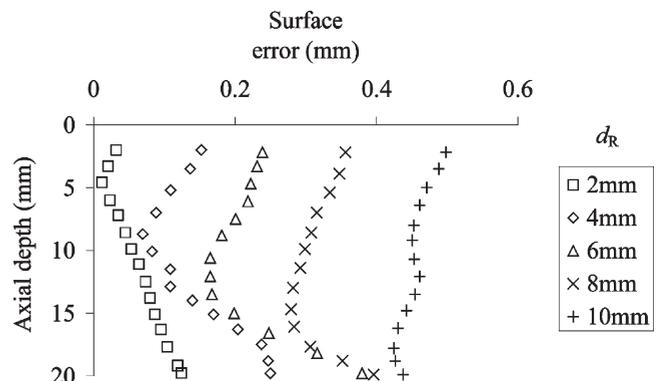
Fig. 2. Errors in down milling with increasing radial depth of cut ( $d_A = 20$  mm,  $F = 200$  mm/min,  $N = 400$  rpm).
