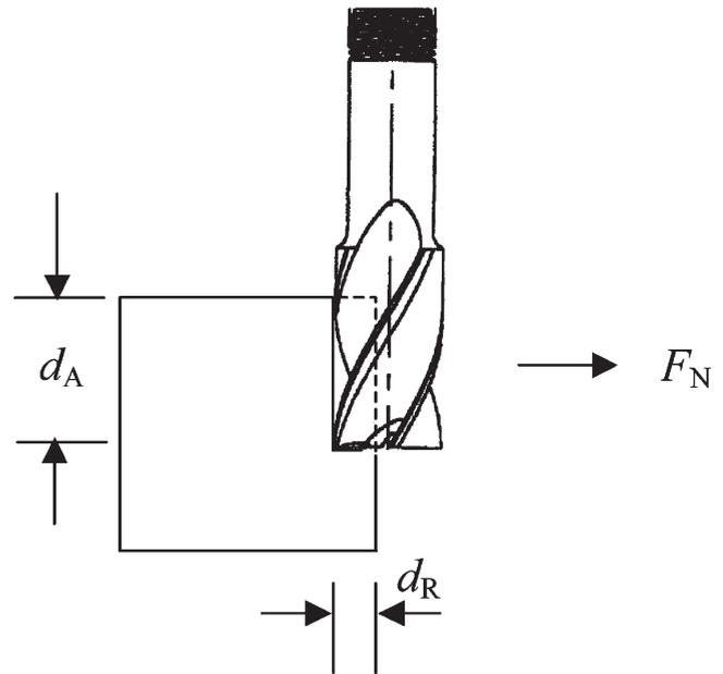
Fig. 1. Side view of end mill in cut.
