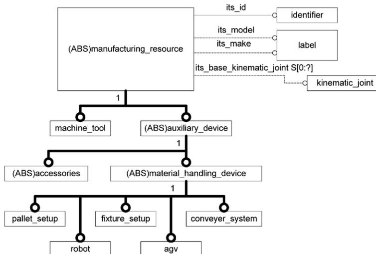
Fig. 2. EXPRESS-G diagram of the manufacturing resource model.
