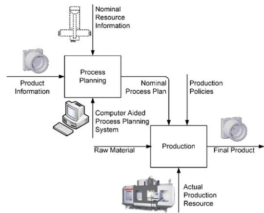
Fig. 3. IDEF-0 representation of the state of the art in process planning.
