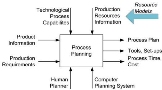
Fig. 1. IDEF-0 diagram for the process planning activity, adapted from [1].
