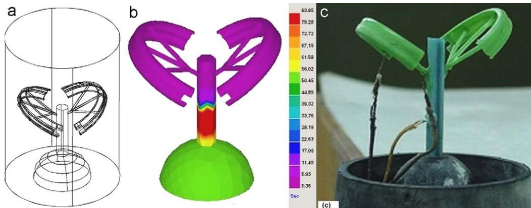
Fig. 1. Examples of investment casting artefact (a) mould model (b) solidification time distribution (c) wax tree.
