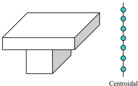
Fig. 2. Centroidal axis fails to detect the geometric change.
