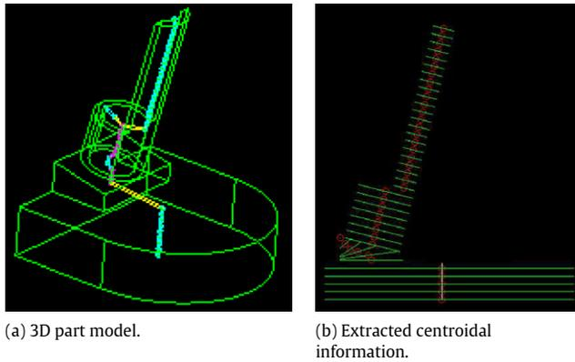
Fig. 1. Example of centroidal axis extraction of CAD model.
