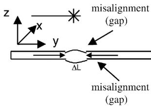
Fig. 3. In-plane shrinkage.
