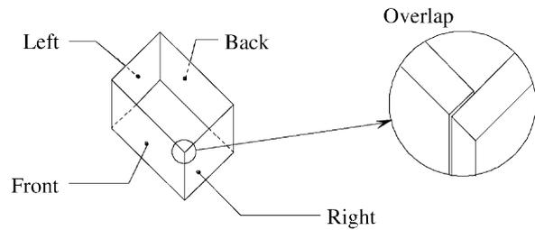
Fig. 4. Simple sheet metal box.
