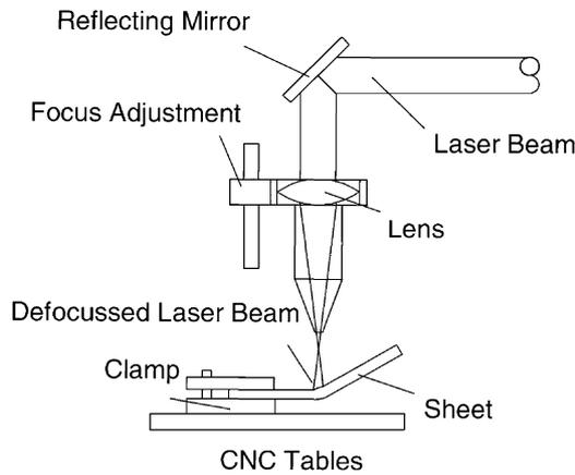
Fig. 1. A laser forming set-up.
