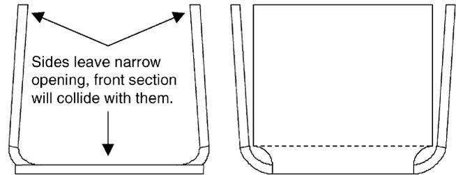
Fig. 5. Collision danger (left) and unwanted gap (right).
