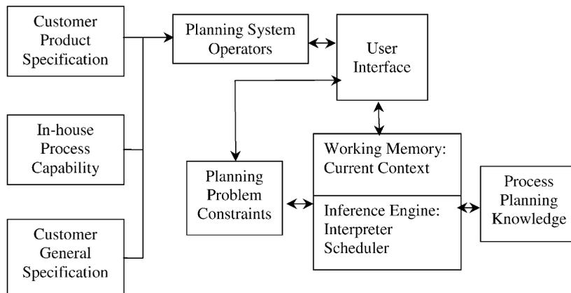
Fig. 1. Architecture of knowledge-based CAPP system.
