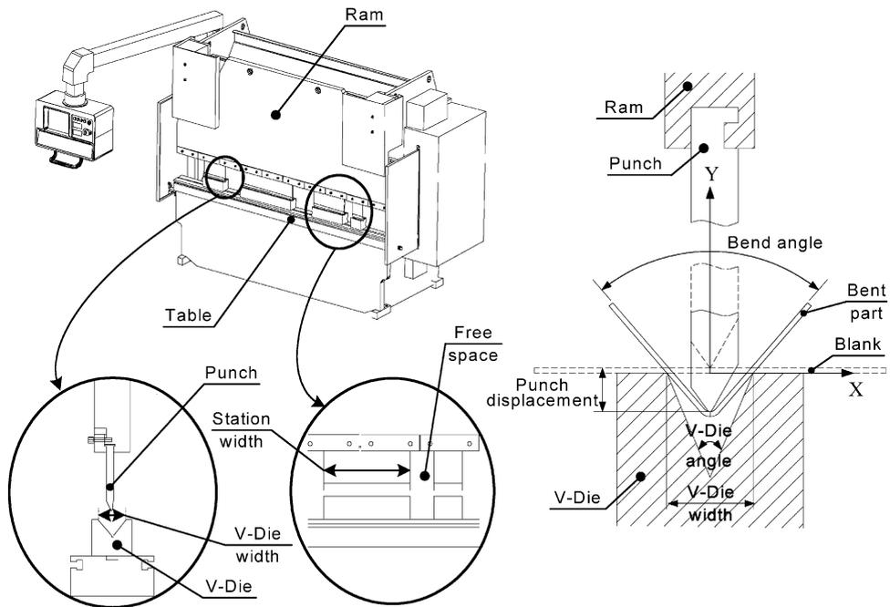
Fig. 1. The bending process and its resources.
