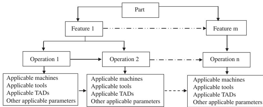
Fig. 1. Representation of a process plan.
