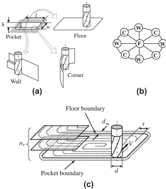
Fig. 1. Representation of 2½D pocket in terms of: (a) elemental machining surfaces; (b) adjacency graph; and (c) Floor.
