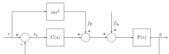
Fig. 2. Block-diagram representation (with  $s$  the Laplace variable) of a simplified position tracking control scheme for the short-stroke reticle stage module in scanning direction.
