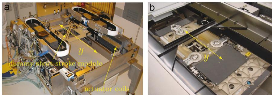
Fig. 1. Long-stroke (left) and short-stroke (right) reticle stage modules of an industrial wafer scanner: (a) long-stroke reticle stage module, (b) short-stroke reticle stage module.
