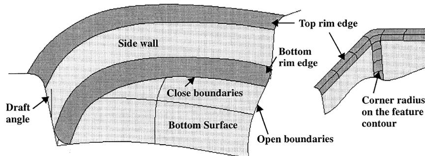
Fig. 1. A typical freeform surface feature.
