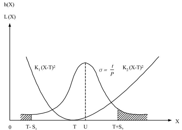
Fig. 1. Relationship between the design target  $T$ , design tolerances  $S_1$  and  $S_2$ , process mean  $U$ , and process tolerance  $t$ .
