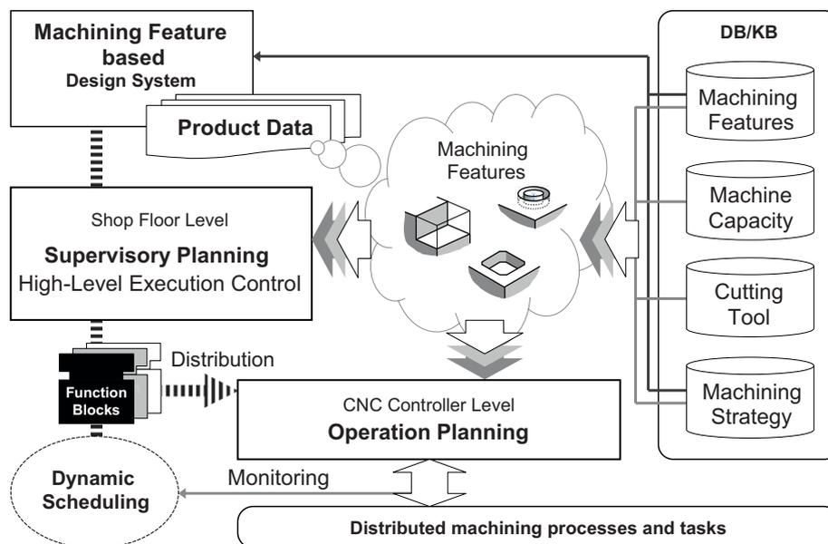
Fig. 2. Concept of distributed process planning.
