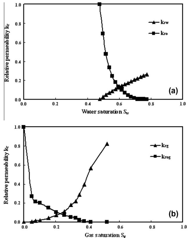
Fig. 1. Typical relative permeability curves for the target oil reservoir. (a) Relative permeability curves for water–oil system. (b) Relative permeability curves for gas–liquid system.
