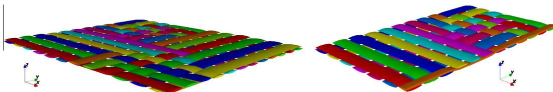
Fig. 1. The unit cell geometry used by Ilyani Akmar et al. [24]: (left) an elementary pattern; (right) the half of elementary pattern.
