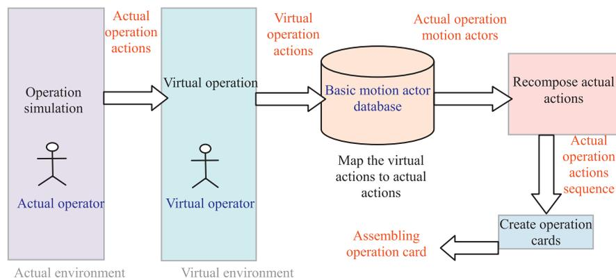
Fig. 1. The process of assembling operation process planning based on interactive operation simulation.
