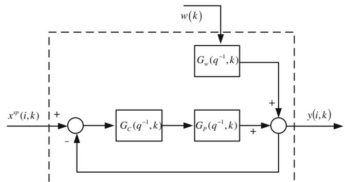
Fig. 1. Block diagram of feedback control for the batch system.
