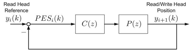
Fig. 2. Block diagram of Self-ServoWriting servo loop.
