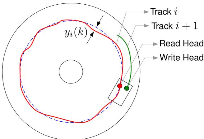
Fig. 1. An illustration of Self-ServoWriting process.
