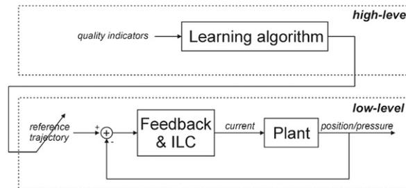
**Fig. 2.** The applied two-level control scheme with a low-level ILC controller and a high-level learning algorithm to update the reference of the low-level controller.
