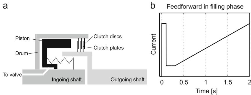
**Fig. 1.** A wet clutch: (a) the mechanical design and (b) the typical feedforward current signal to the electro-hydraulic valve in the filling phase.
