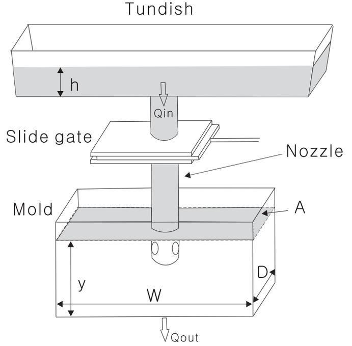
Fig. 2. Tundish and mold.
