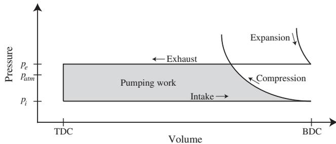
Fig. 1. Schematic indicator diagram showing pumping work (shaded).
