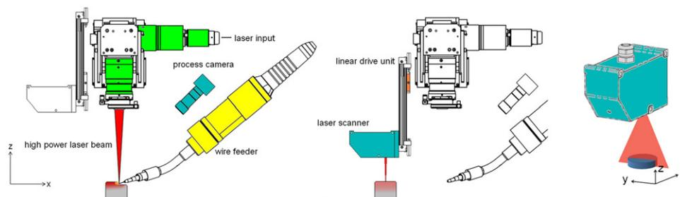
Fig. 1. Deposition tool with the laser scanner. Left, deposition mode; middle, scanning mode; right, coordinate axes during scanning.
